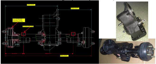
In production since 2007 – Ratios – 18:12, 15.42, 14.67, 13.13, 12.49, 11.48, 10.25, 8.32, 7.75, 6.47 & 5.24 – (19) tooth input spline only, open differential – optional limited slip. Design can be used as independent or with axle & axle housing. 94.45lb.ft. Maximum input torque. Axle housings are wet. Many widths available and upgrade axle capacity – standard 1800 lb max to 3500 lb. With optional bearings
