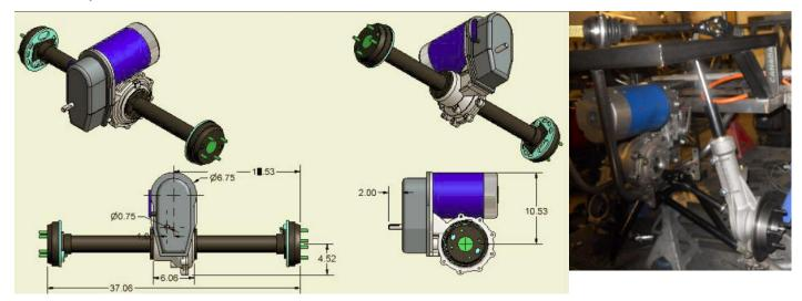
In production since 2009 – Ratios – 12.5 & 20.0 or 12.5 & 16.0, 19 tooth input spline only, open differential. Design can be used as independent or with axle & axle housing. Self contained center gearbox, 100lb.ft. Maximum input torque. Axle housings are dry. Many widths available
