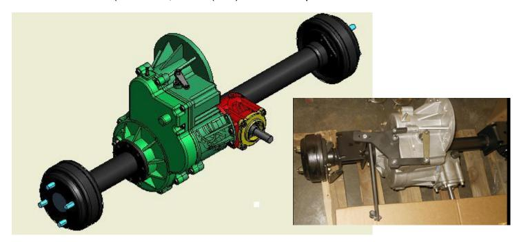
In production since 2011 – Ratios – 10.0 & 20.0, 19 & 10 tooth input spline or 17.0 & 24.0, 19 & 10 tooth input spline - open differential with manual differential lock or limited slip. Design can be used as independent or with axle & axle housing. Self contained center gearbox, 130lb.ft. Maximum input torque. Axle housings are dry. Many widths available, 4x2 or 4x4 capable
