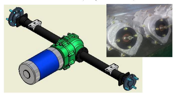
In production since 2012, ratio 20.00:1, with open diff, locking axle – 10 or 19 tooth input, – center gearbox is self contained and axle housings are dry. Many widths available
